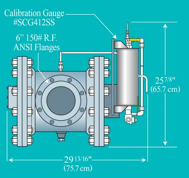
The **Model 1000** is designed to handle the **high gallons per minute flow rates** associated with **bulk fuel receipt**.
